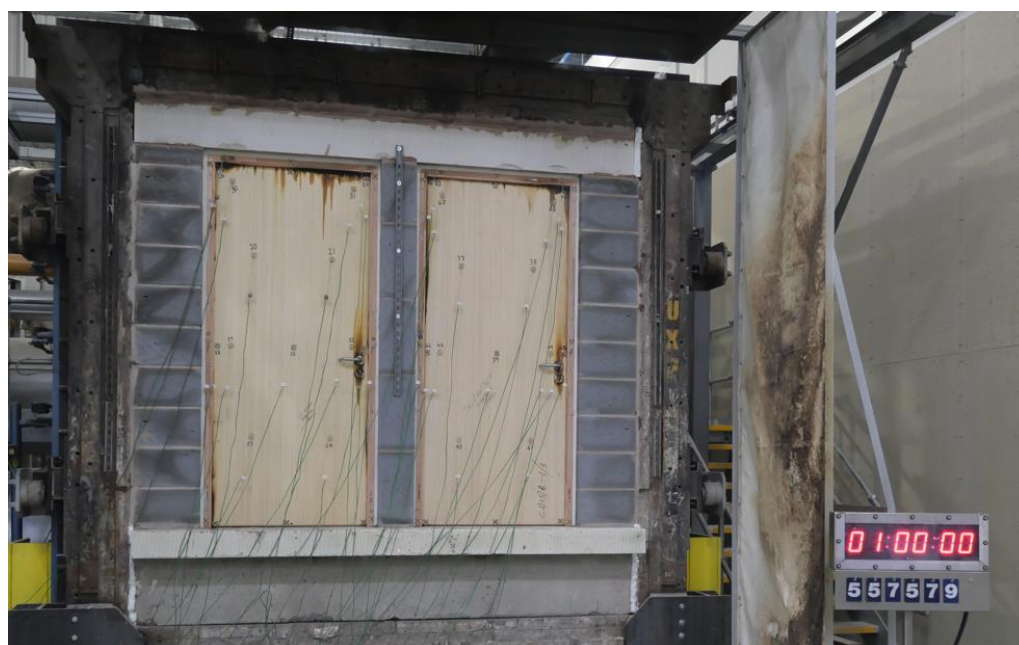
The unexposed face of the specimens after a test duration of 60 minutes
