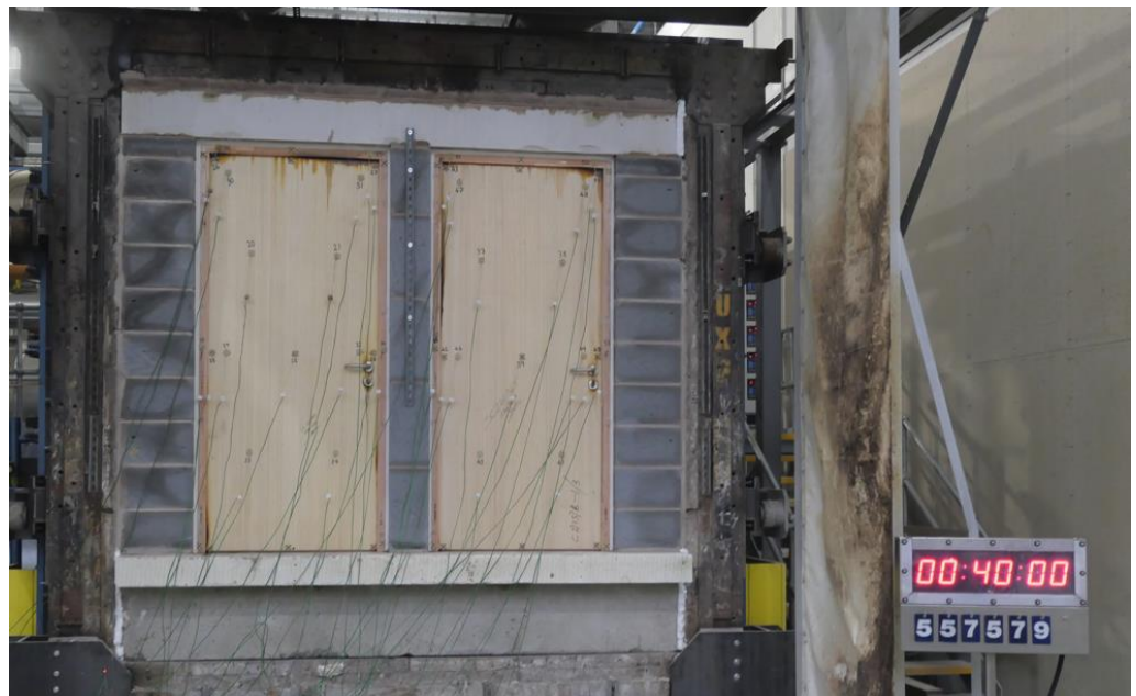
The unexposed face of the specimens after a test duration of 40 minutes
