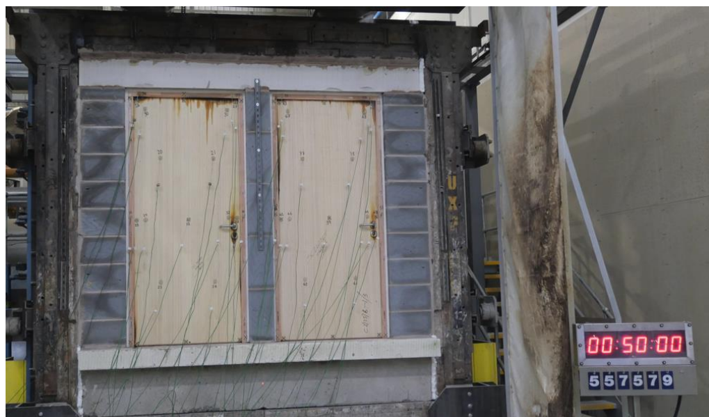
The unexposed face of the specimens after a test duration of 50 minutes
