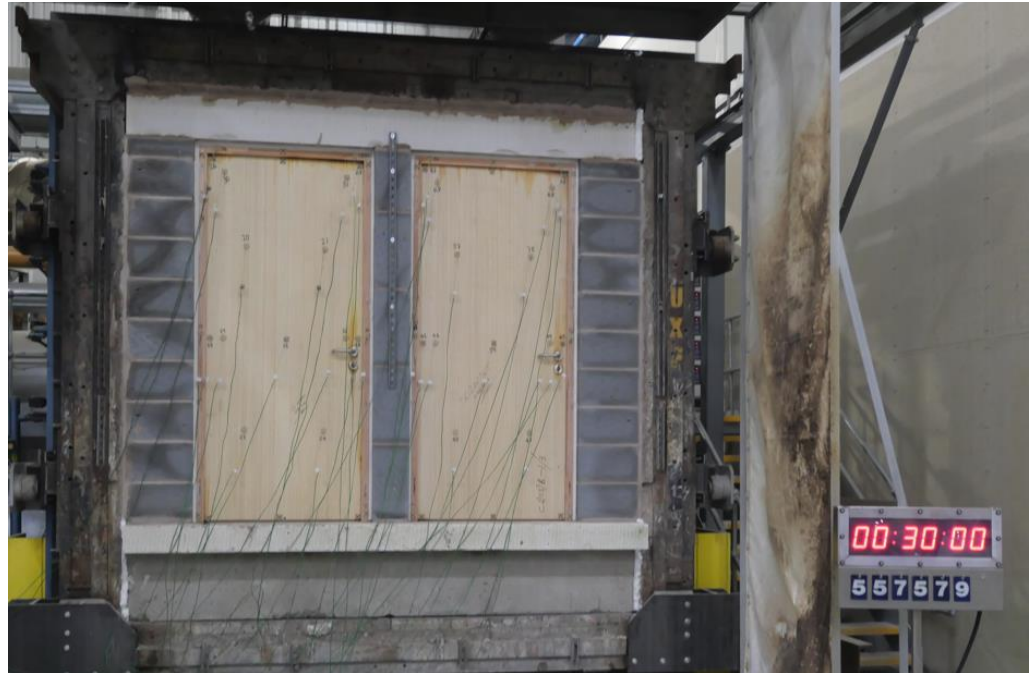
The unexposed face of the specimens after a test duration of 30 minutes
