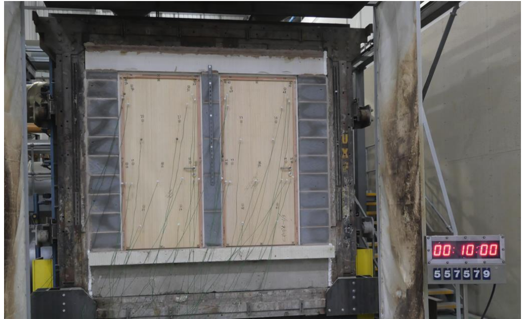
The unexposed face of the specimens after a test duration of 10 minutes
