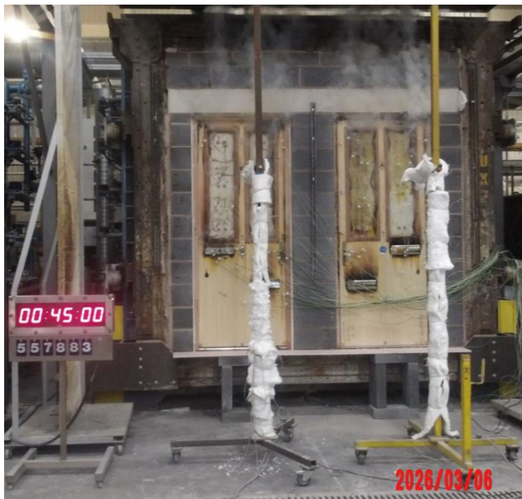
The unexposed face of the specimen after a test duration of 45 minutes
