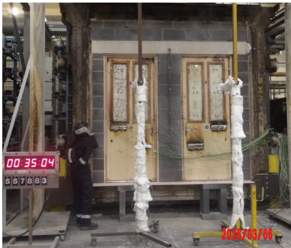
The unexposed face of the specimen after a test duration of 35 minutes
