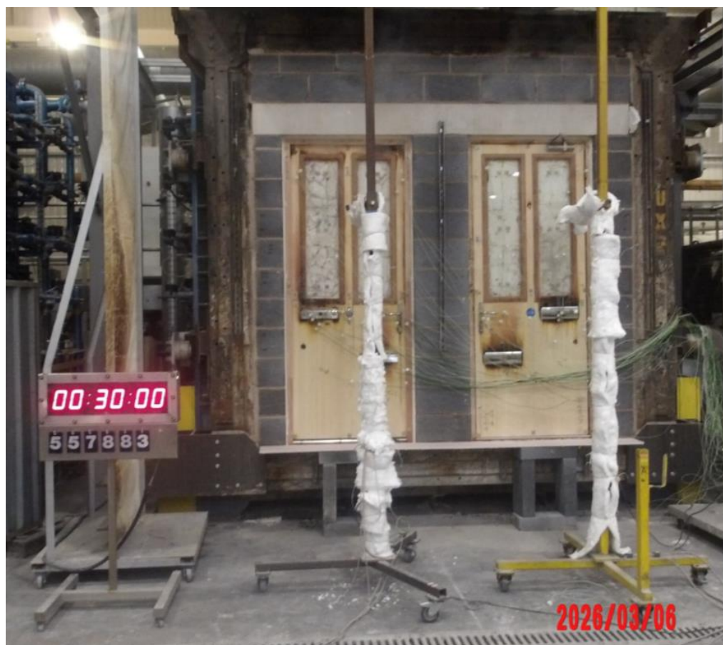
The unexposed face of the specimen after a test duration of 30 minutes
