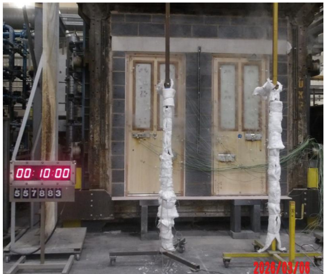
The unexposed face of the specimen after a test duration of 10 minutes
