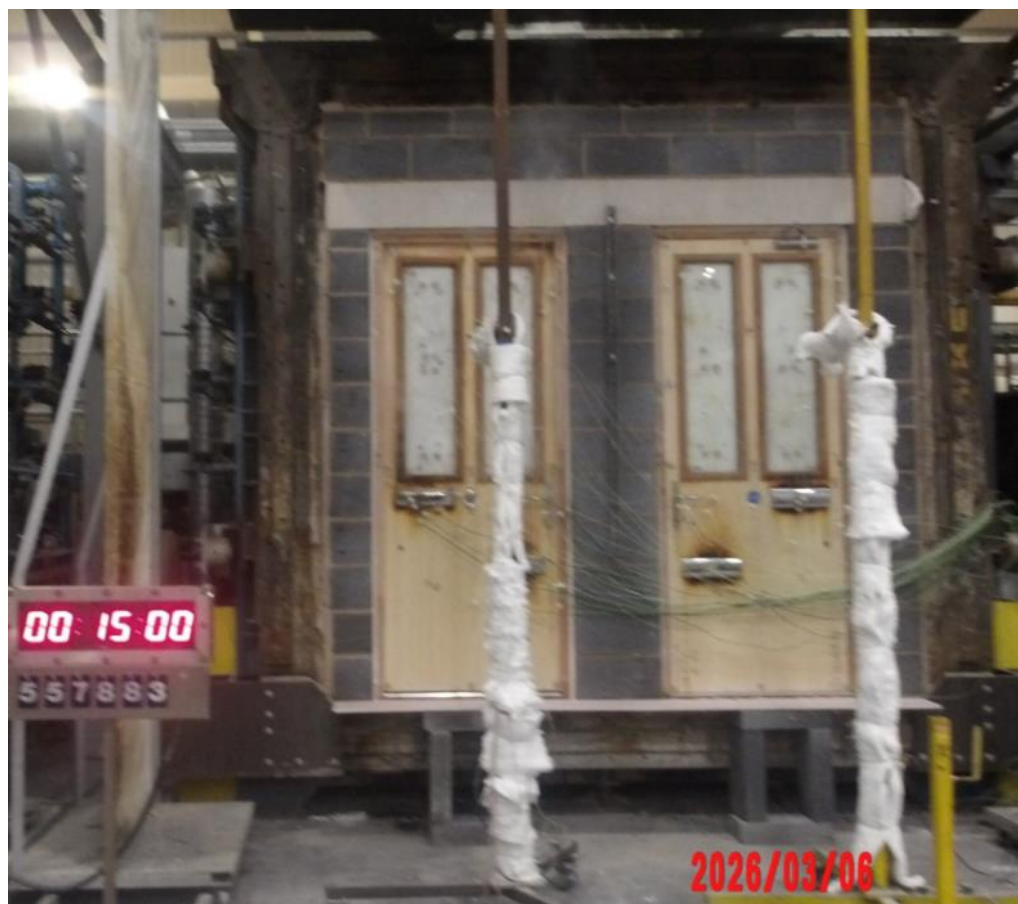
The unexposed face of the specimen after a test duration of 15 minutes
