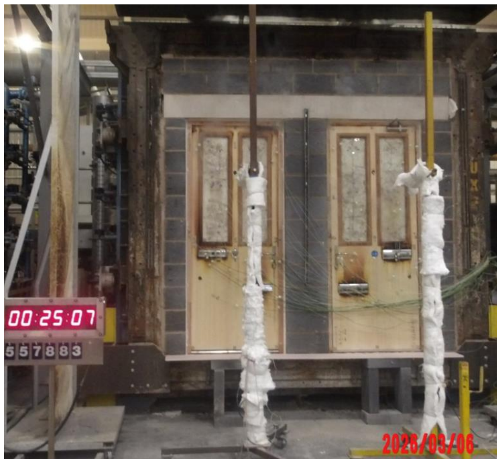
The unexposed face of the specimen after a test duration of 25 minutes
